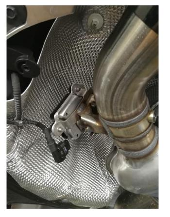
Remove OE Connector from actuator and fit Module connectors between OE Connector and actuator
