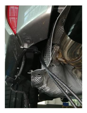
Fix shorter Harness connector to Valve under the Cable gland and longer to the opposite side
