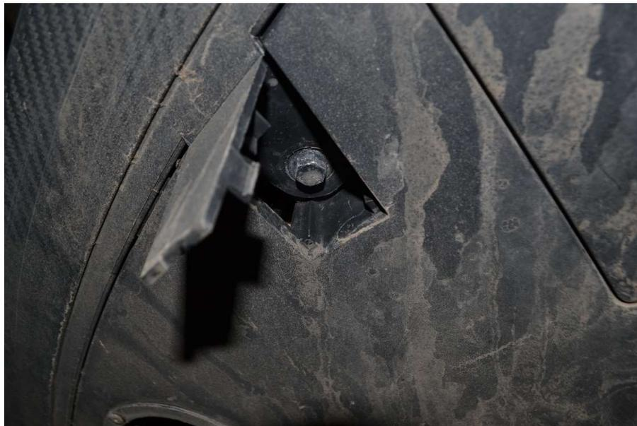
5. Now remove the plastic rivets holding the wheel arch liners to the bumper and undertray, these run inside the wheel arch and to the back of the under tray
