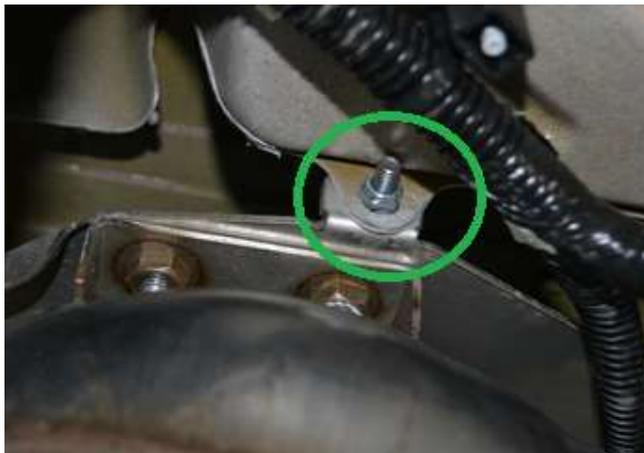
13. The final bolt is fitted to the chassis rail, the mounting plate supplied is slide inside the rail and the final M8 x 16mm bolt fixes through the bracket and chassis rail to securely hold the sound generator in place
