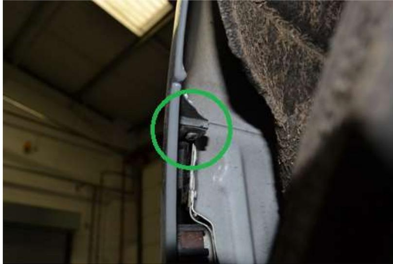
7. Starting on the left-hand side (as you are looking at the vehicle) slowly unclip the bumper cover to gain access to the rear parking sensor connector housing to enable this to be disconnected
