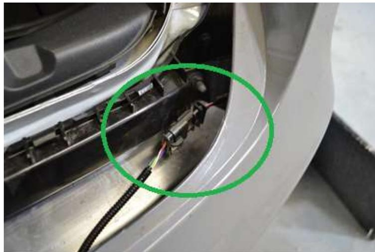
8. Now the bumper cover and under tray can be fully removed from the vehicle, place this on a soft surface and ensure it cannot fall and cause damage to the cover.
