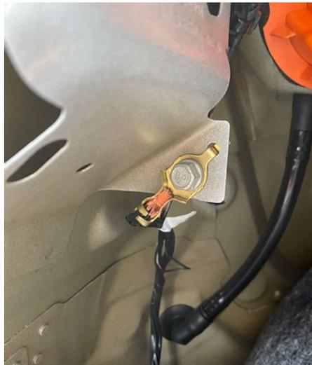
23. The remaining pair of cables, Red 12v switched live feed and the CANBUS twisted pair now need to be run along the side of the vehicle behind the trunk side carpet up and over the wheel arch.
