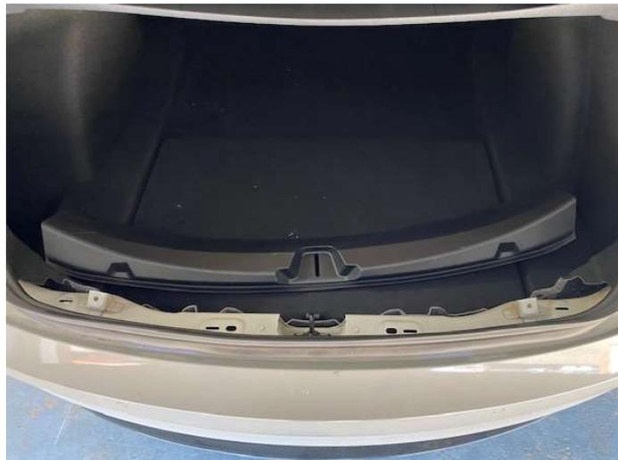
2. Loosen the rubber seal on either side of the trunk area and unscrew the top retaining screw on each of the rear taillight.
