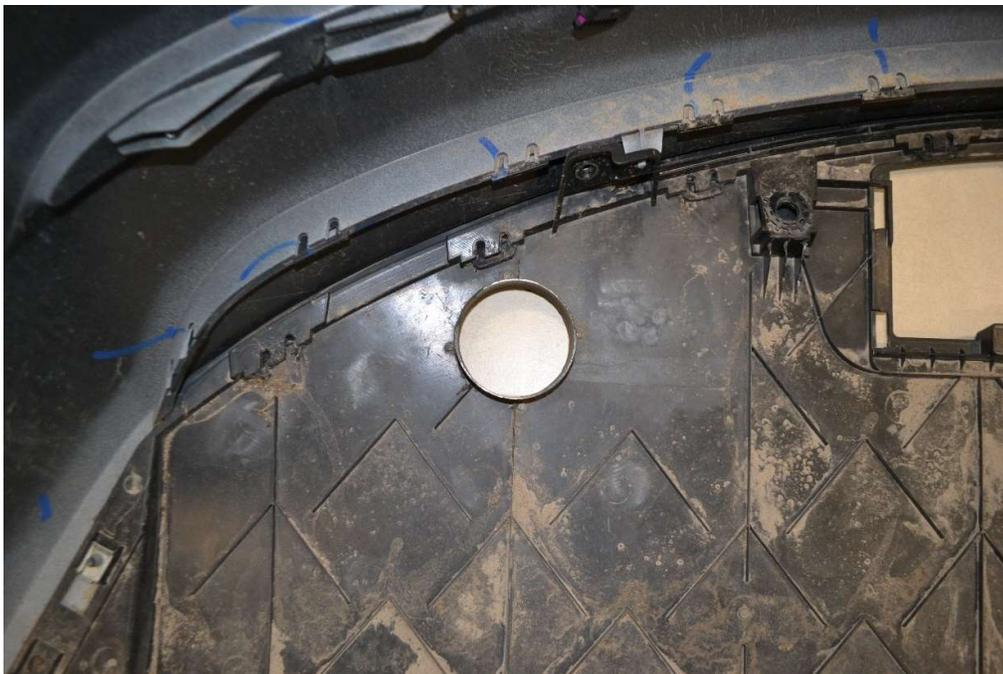
18. De-burr the hole cut into the plastic undertray and now from the underside insert the trim finisher and fix to the plastic with the 4 self-tapping plastic screws
