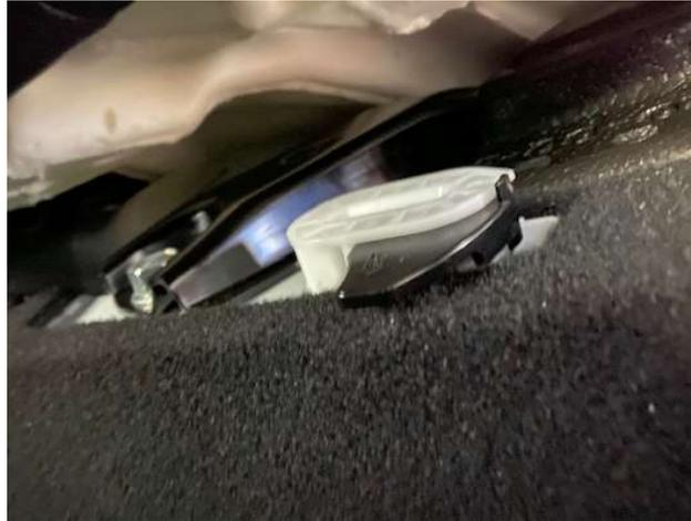
25. Pull the seat cushion base up and out to remove and safely place to one side.
