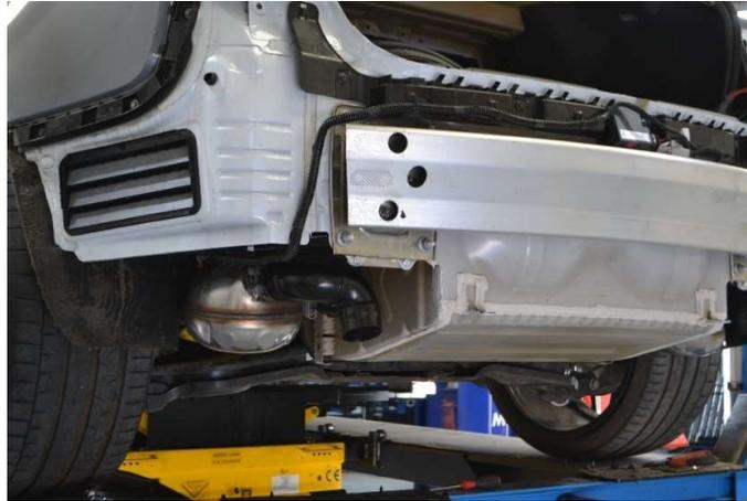
11. Two M8 x 16mm bolts are used to secure the rear of the bracket to the open holes in the back of the plate for the crash bar
