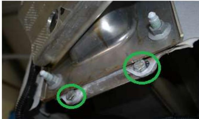
12. The M6 bolt, washer and nyloc nut are used for the side hole of the bracket to the body of the vehicle
