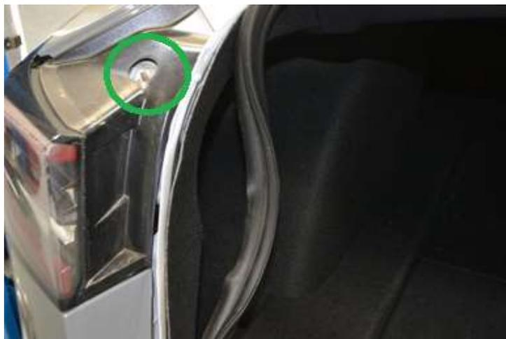
3. Complete the removal of the taillight by disconnecting the electrical connector and removing the nut on the inside securing the light unit and put the light units to one side safely.
