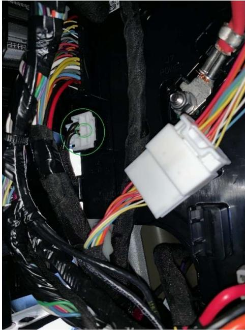
35. If no wire is present connect the 5mm spade connector on the provided loom directly to the pin on this empty slot of the VC-LEFT connector and secure the cable, if the red wire is present trace this down to the main loom, remove the spade connect on the provide loom and connect to the red wire using the supplied POSI-Lock connector.
